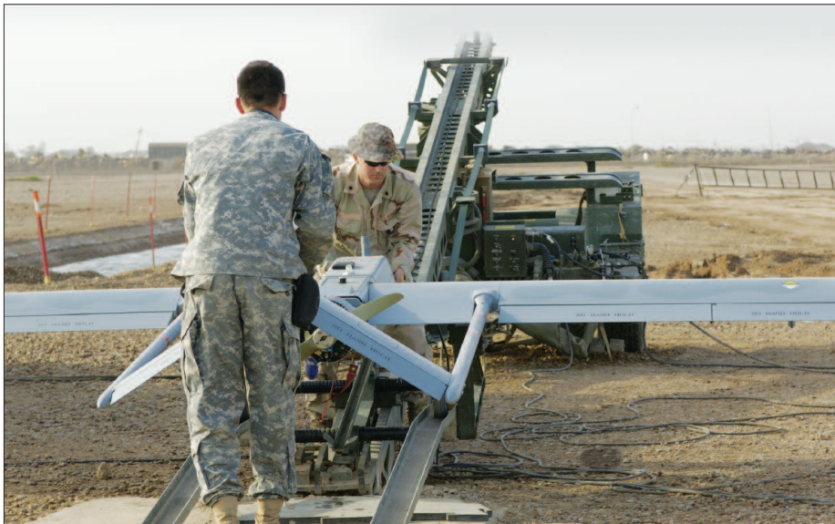
A ground crew can prepare a launcher and ready a Shadow 200 aircraft for flight in a matter of minutes. The hydraulic launcher mounts on a standard, high-mobility trailer.
