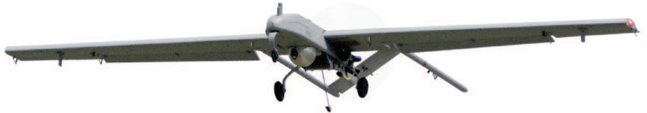
The Shadow 200 aircraft has been enhanced with extended wings for superior endurance.
